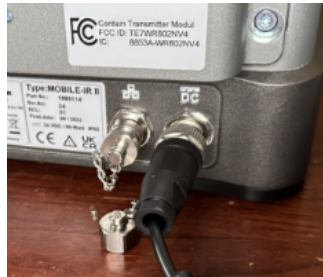
Figure 35. Charging port (left) net to Ethernet port (right).
