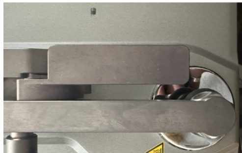
Figure 31. Larger lever even with the anvil. (Best position for scanning).
