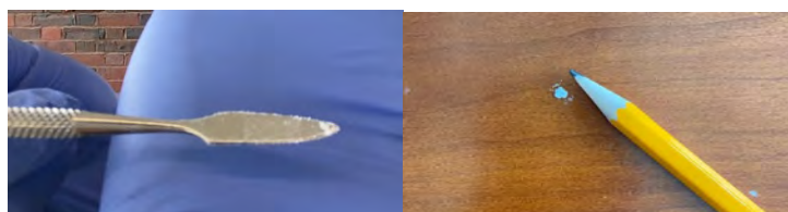
Figure 28. Visualize one (1) milligram of sample.
