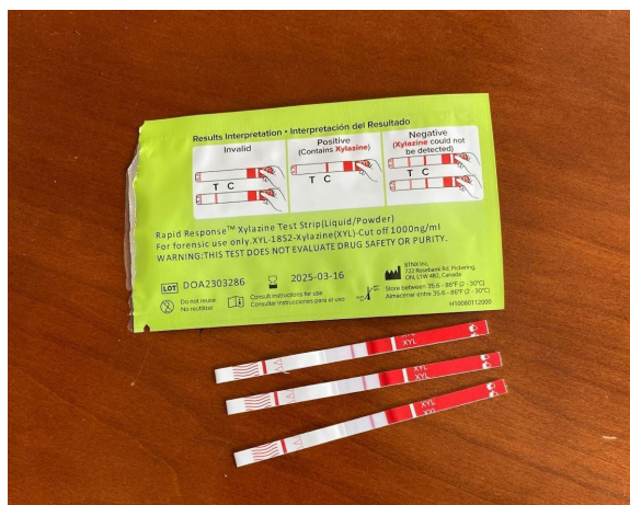
Figure 31. Interpretation of Xylazine Test Strip Results.
