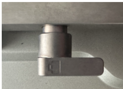
Figure 32. Smaller lever in transportation position (level with the Anvil).
